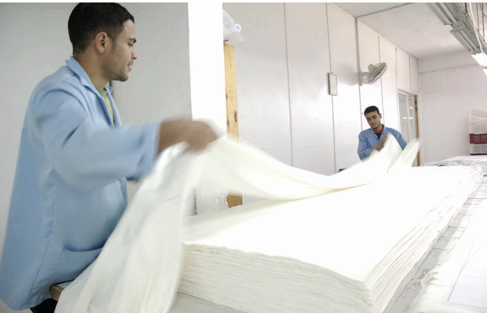
All fabrics used in the cutting department have been organically produced. Here they are laid out on the table for cutting the single pieces of the garments according to the patterns.
